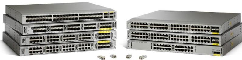
The Cisco Nexus 2000 Series provides two types of ports: ports for end-host attachment (host interfaces) and uplink ports (fabric interfaces). Fabric Interfaces are differentiated with a yellow color for connectivity to the upstream parent Cisco Nexus switch.
