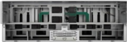
Figure 2. Cisco UCS S3260 (empty chassis)
