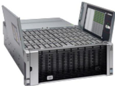
Figure 1. Cisco UCS S3260 Storage Server
